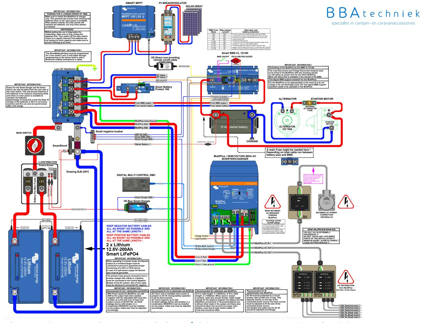
US-VAN Drawing Smart BMS CL12/100 MultiPlus 3KW DMC 400Ah Li VEBus Smart Dongle & Shunt SBP 100A MPPT 100/50
