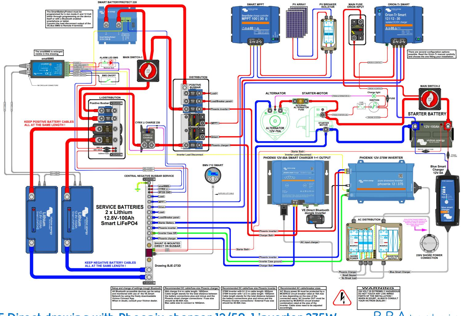
VE.Direct drawing with Phoenix charger 12/50-1 inverter 375W Li Batt smallBMS MPPT 100/30 Orion-Tr Smart
