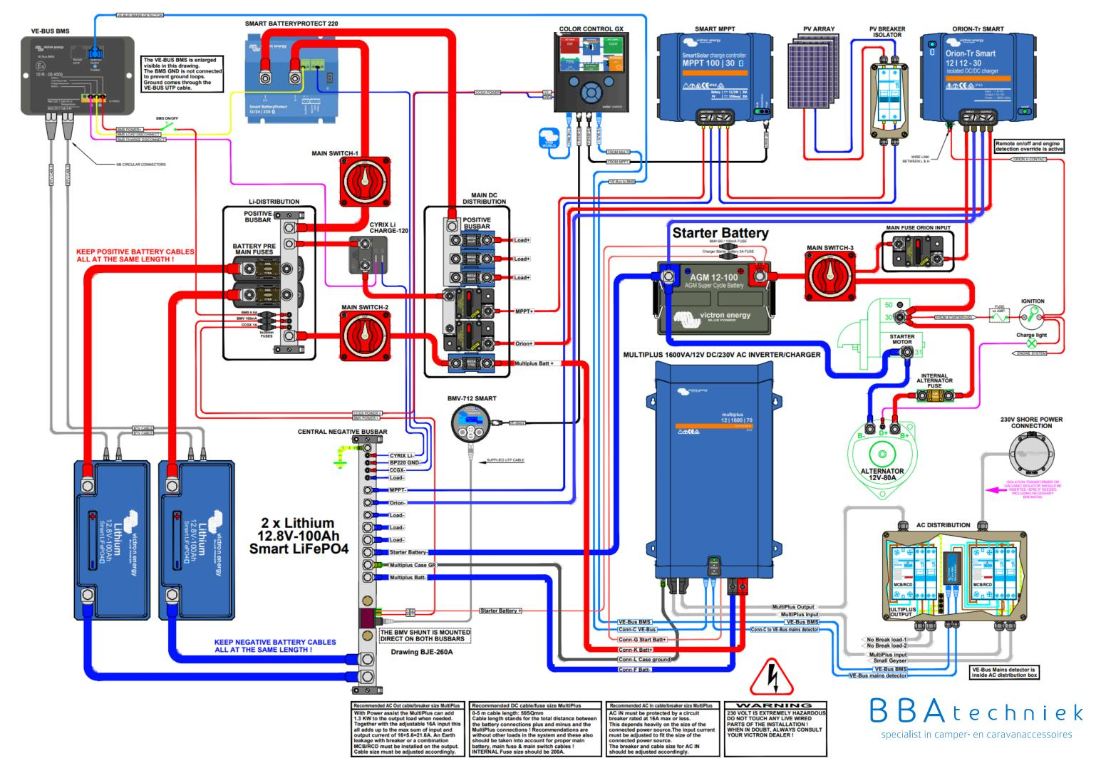
1.6kVA 12V MultiPlus 230 Volt system example 4 PIN VE-Bus BMS-Lithium Orion-Tr
